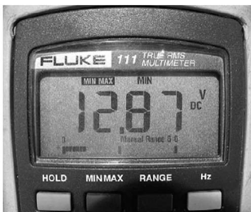
If the electrical system cannot sustain at least 12 VDC, check the following:
