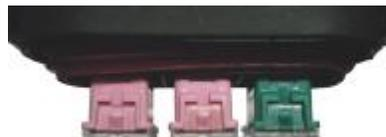
1. To remove fuse box cover, simultaneously squeeze tabs inwards on each end of fuse box cover as you pull downward on the cover.
